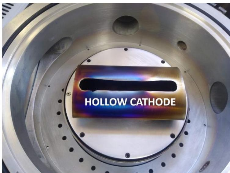
**Figure 4.10.** Photograph of the interior of the hydrogenation chamber with the hollow cathode positioned.
